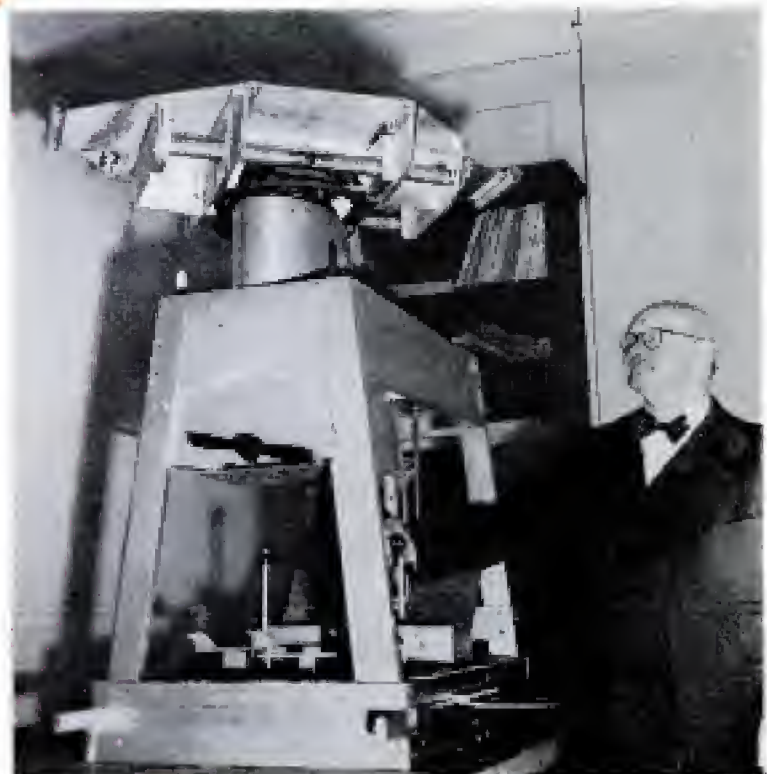
Mockup of convertiplane in Herrick's office is equipped with complete controls, revolving rotor head and forward propeller
